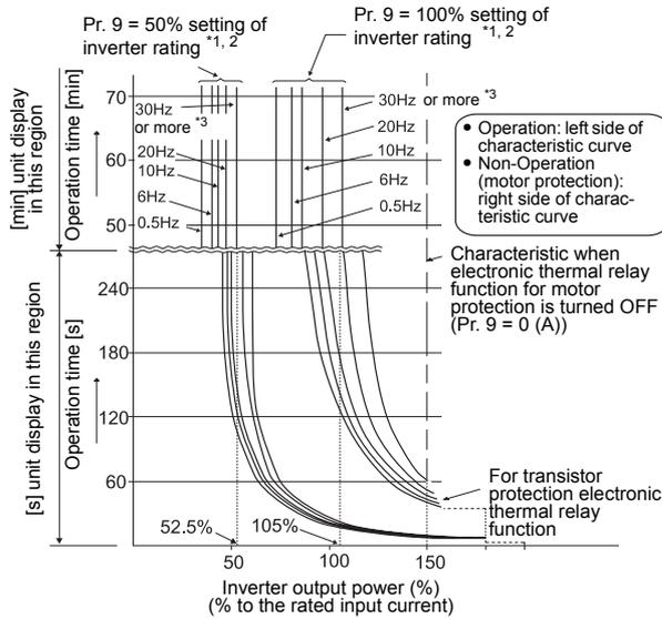
This function detects the overload (overheat) of the motor, stops the operation of the inverter's output transistor, and stops the output.
