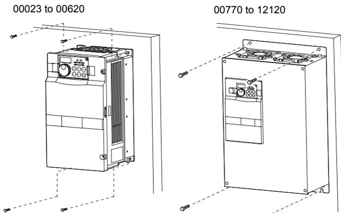
Fix six positions for the FR-A 740-04320 to 08660 and fix eight positions for the R-A 740-09620 to 12120.
