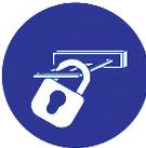
Before beginning the visual inspections or cleaning tasks, switch off the main switch(es) and secure them from being switched on again using a padlock.
